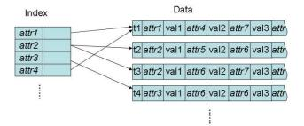
Figure 10: Storage and Index scheme for the generic table.
