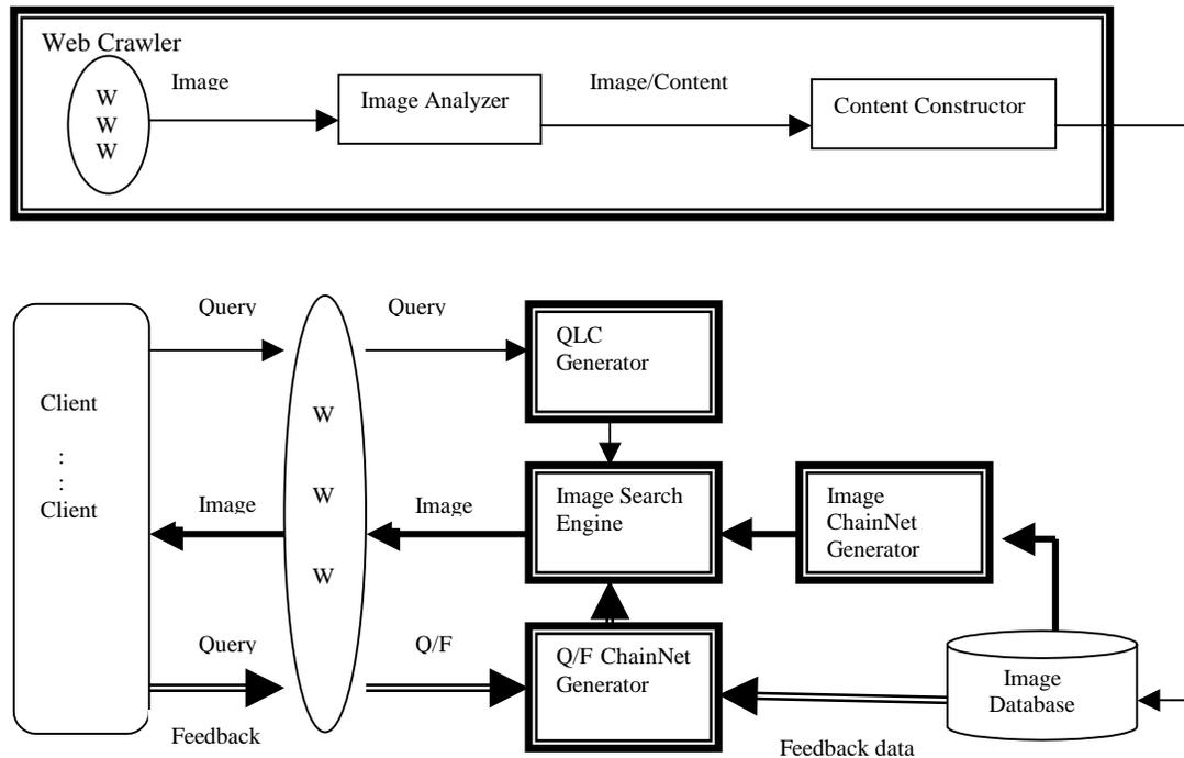
Figure1: Overall system structure in client-server form.
