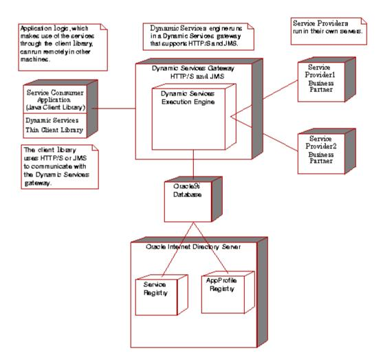
Figure 1–6 Java (HTTP/JMS) Deployment View of the Oracle Dynamic Services Framework
