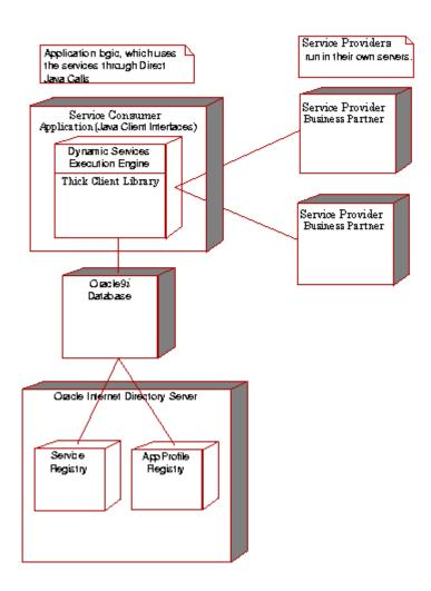
Figure 1–4 Java Deployment View of the Oracle Dynamic Services Framework
