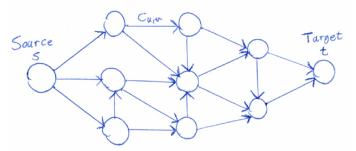
• Let V denote the set of nodes and E denote the set of edges in the graph (i.e.,  $(u, v) \in E$  indicates an edge pointing from u to v), and let s and t denote the source and target nodes.
