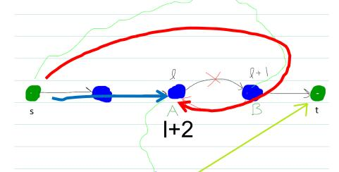
So, from the time edge (**A**, **B**) is the bottleneck edge, deleted due to an augmenting path, and reappears later, dist(**s**, **A**) <u>must have increased by at least 2</u>
