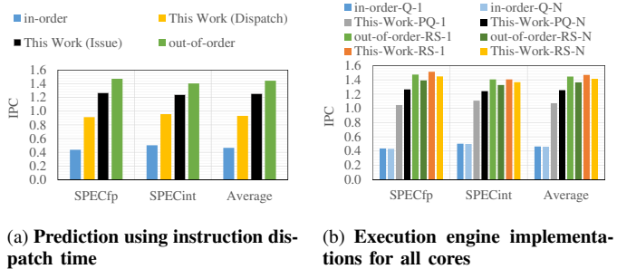
Fig. 8: Implementation options for (a) the prediction algorithm and (b) the execution engine (Q and PQ: issue from the head, RS: issue from any position in the queue, 1: one instruction queue for all units, N: one queue per functional unit).
