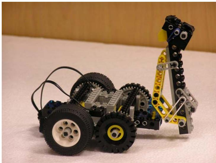
Figure 5: Attaching the pen holding arm to the driving base
