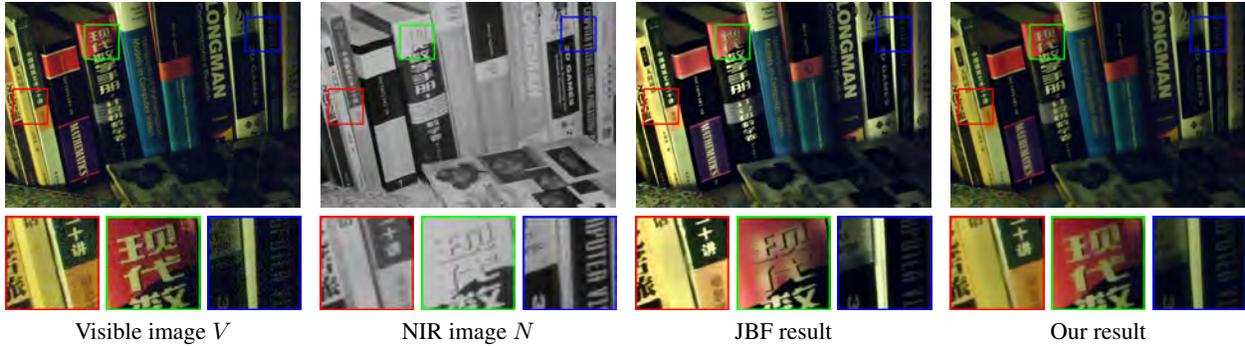
**Fig. 4.** Comparison of our method with joint bilateral filtering (JBF). Our method can avoid color shift, edge blur and halo problems that JBF suffers from.
