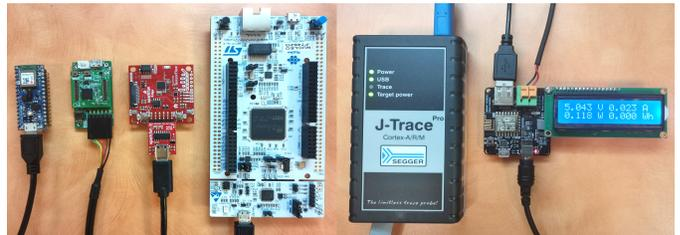
Fig. 1. Picture of Arduino Nano 33 BLE Sense, Nucleo-64 STM32L476RG, SparkFun Edge Apollo3 Blue, Nucleo-144 STM32F746ZG, J-Trace Pro Debug Probe, and SmartPower2 (from left to right).
