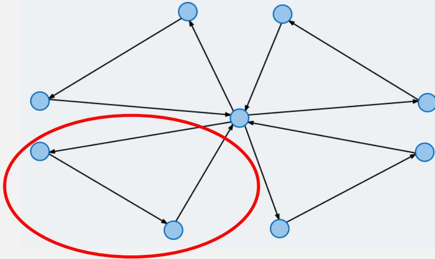
A subtour  $a \rightarrow \alpha \rightarrow a$  can be integrated into the main tour  $\beta \rightarrow a \rightarrow \gamma$  by inserting it as  $\beta \rightarrow a \rightarrow \alpha \rightarrow a \rightarrow \gamma$
