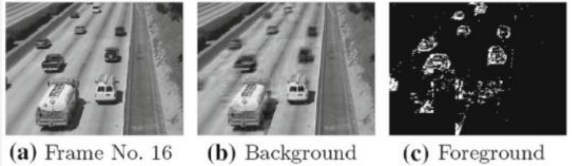
Fig. 6 Modeled Background and detected Foregrounds using 10 strongest eigenvectors
