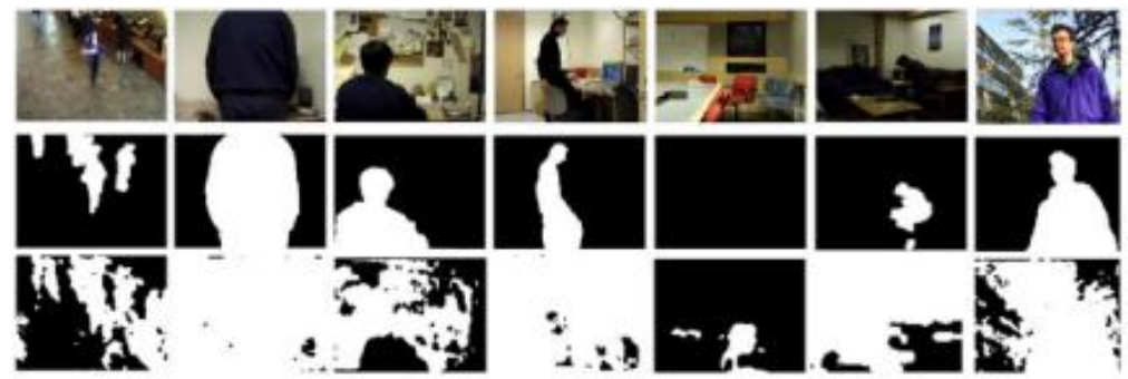
Fig. 1 The result of the Eigenbackground (Fig. 9 of [19]) in background modeling. From top to bottom, the original images, ground truth and the results of foreground detection using background models created by the Eigenbackground method (courtesy from [19])
