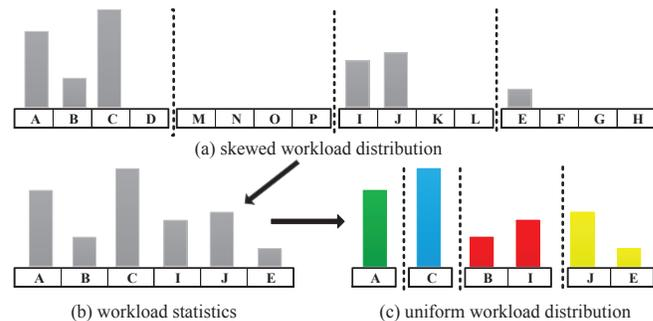
Fig. 3. Dynamic partitioning based on actual workloads.
